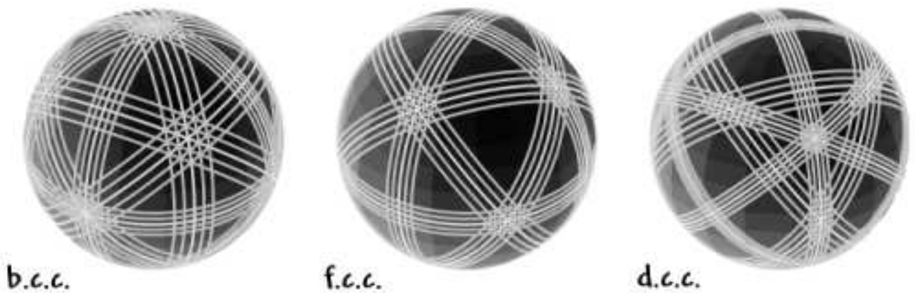
FIG. 6: Visibility maps for the two largest fringes visible from body-centered, face-centered, and diamond face-centered lattices. Sphere diameter (relative to band width and fringe spacing) is proportional to specimen thickness, here chosen to be about 5 times the cubic cell side a . Note the dominance of crossed \{110\} fringes at the three-fold \langle 111 \rangle zone in the body-centered case, the dominant crossed \{111\} fringes at the two-fold \langle 110 \rangle zone in the face-centered cases, and the wider disparity between largest and next-to-largest spacings when the diamond glide is added to the lattice.
